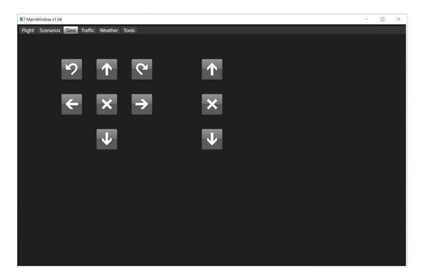
The slew page allows for the glider to be moved around geographically both laterally and vertically.
